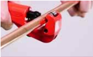
1. Cut the tube to length
